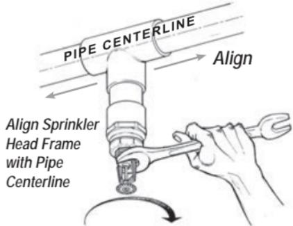
**NOTICE** Back-up wrench may be applied to the Adapter flats for removal of sprinkler head if required.
